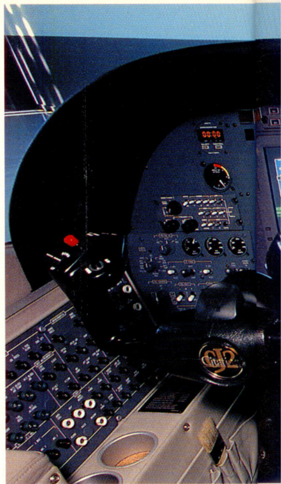
The standard CJ2 panel includes a single PFD and MFD; a copilot's PFD is a popular option, though—even with its $118,000 price tag. Overall, the CJ2 airframe is larger than its predecessors, with its bigger engine nacelles and swept horizontal stabilizer being the quickest ways to single out a CJ2 on the ramp.
